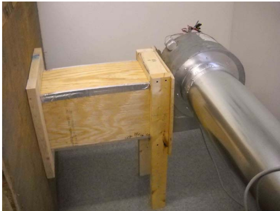
Fan mount on back side of test chamber.
