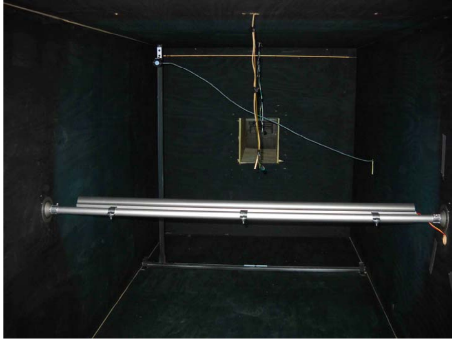
View of test chamber with Sanuvox fixture mounted and UV sensor in upper left position.
