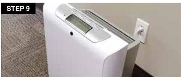
9. **Securely replace the cover:** To replace the unit front cover, first fit the top of the unit into place and slowly press the bottom as to allow the bottom clips to catch.
