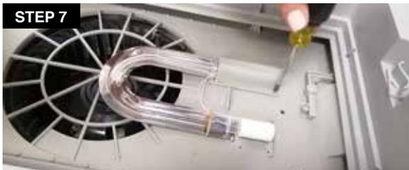
7. **Place the new lamp** in the Biopür and hold it in by **screwing back the gray plastic bracket**. Be careful not to drop the screws in the Biopür.
