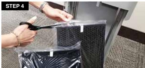
4. **Remove filters from plastic bags** and **replace unwrapped filters** in the following order:
