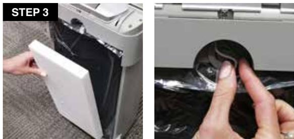
3. Once the Biopür is open, remove the **styrofoam** and discard it. At the top, you will see the locking latch. **Twist latch** to allow the filters to be removed. **Remove all 4 filters.**
