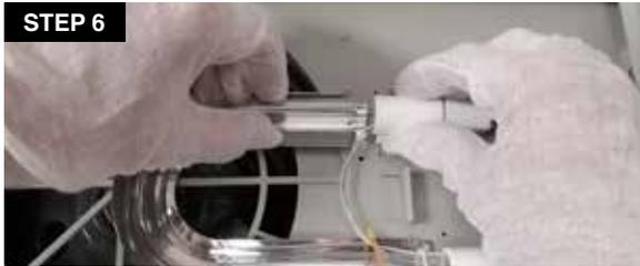
6. Hold the porcelain end-cap (with 4 pins) and carefully push the white connector onto the four pins. The plug is designed so it can only be installed one way. You may have to rotate the socket 90° to line up the pins with the holes. The connector will fit into position.
