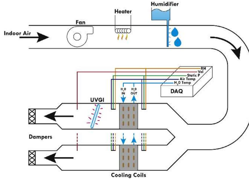
Fig. 1. Schematic of HVAC test apparatus.
