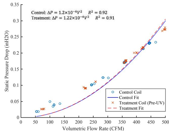
Fig. 2. Static pressure drop versus volumetric flow rate for both cooling coils during the baseline period. The two coils displayed very similar system curves at the start of the experiment. Pressure drop and velocity uncertainty was  $\pm 1\%$ .
