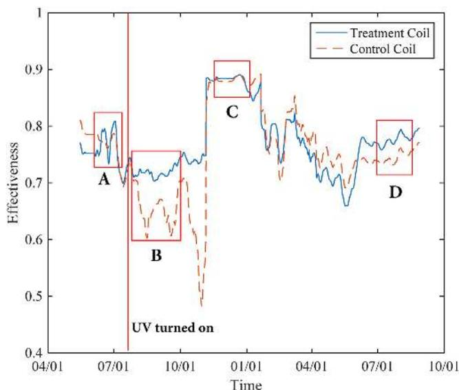
Fig. 3. Time series of calculated effectiveness for UV-treated and control coils over the course of 18 months.
