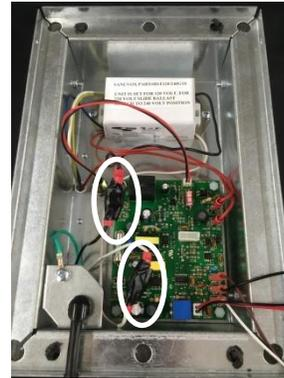
5. Plug the power cord directly in a power outlet and the UV lamp will light up if both the UV lamp and ballast are still functional.
