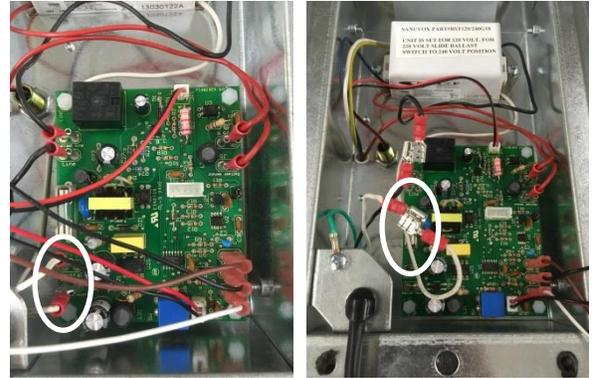
4. Using electrical tape, carefully wrap and cover the 2 connections made in the previous steps
