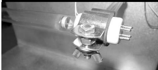
Plug the white-plug onto the UV Lamp's 4 pins. The plug will only fit on in two of four ways. Either way is fine. *The exposed wire-set is Teflon coated and is resistant to UV exposure.*
