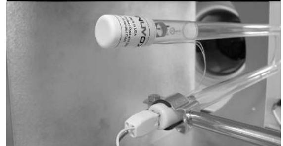
Insert the end-cap with foam gasket into the clamp assembly and tighten. Be careful not to over tighten as you do not want to break the end-cap.
