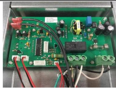
8. Flip the circuit board over so the LCD screen is facing up, making sure no wires are tangled and secure it using the 4 nuts.
