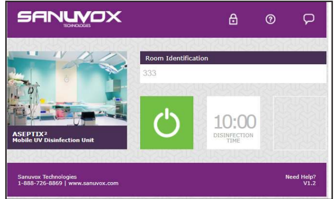
Figure B. Once the "countdown timer" elapses, the ASEPT.2X begins the disinfection cycle which will last 10 minutes.
